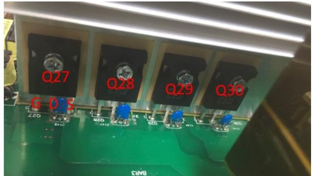
For Axpert Max-7200 ALL of the IGBTs are (IGBT ST/STGW60H65DFB 60A 650V N BULK TO-247)
