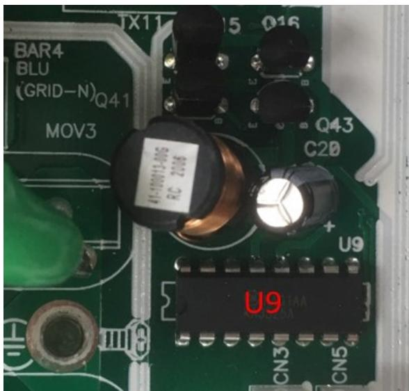
The U9 is (IC PWM CNTL ON/KA3525A)
